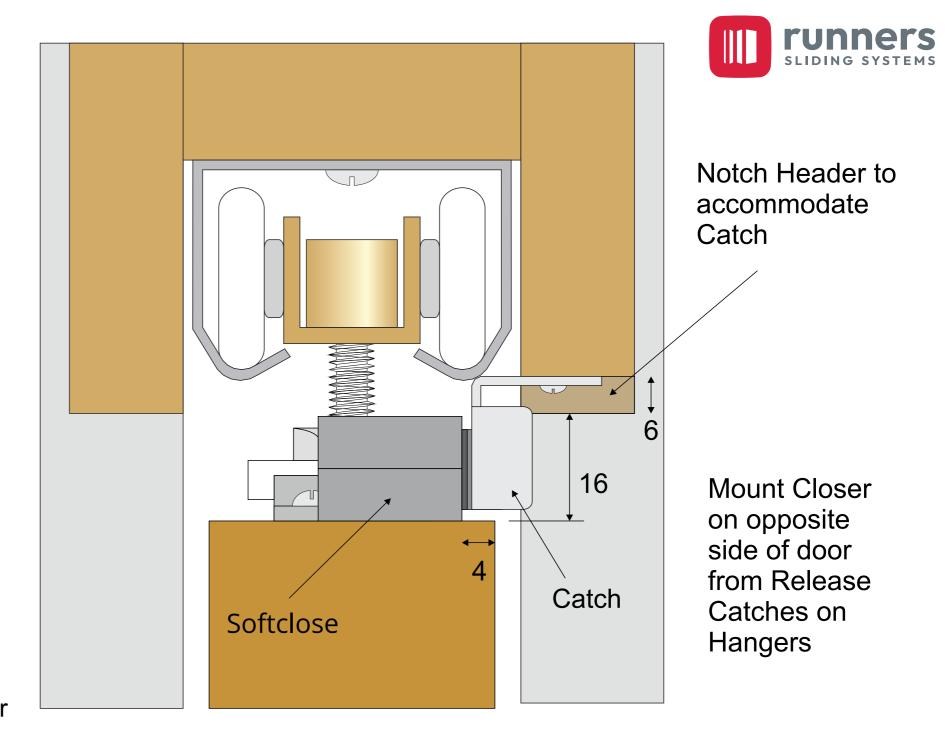
Plan View Showing Top Of Door & Hardware Positioning
